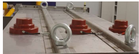
Figure 28 - Bushing of the capacitive divider and example of connection of the busbar voltage detector
